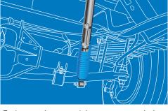
Feature a unique monotube gas-pressure design that provides optimum ride quality and vehicle control: Bilstein shock absorbers last 2-3 times longer than the conventional twin-tube piston and are found in many high-end luxury vehicles
